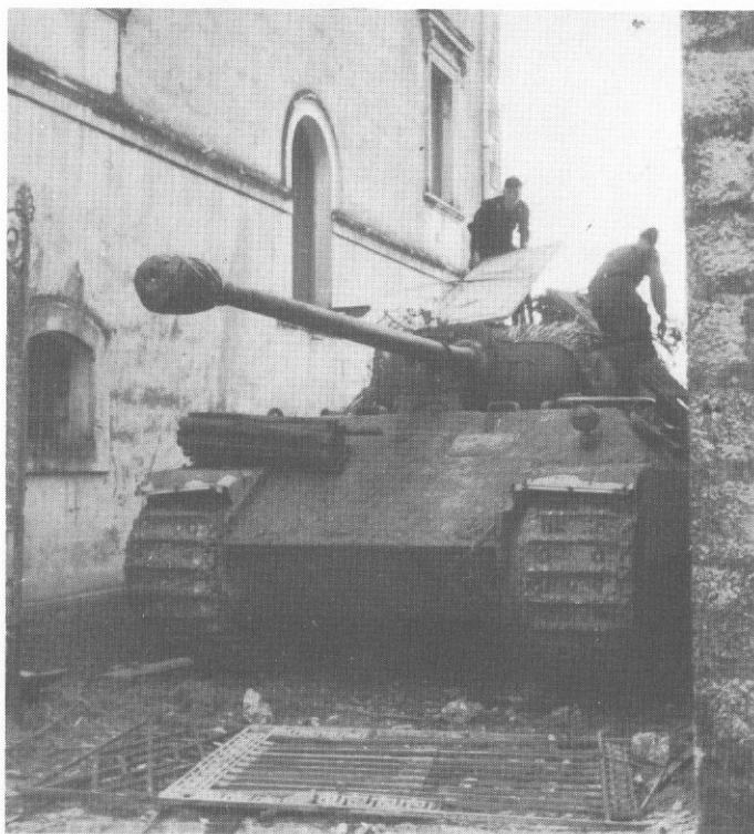
These pages Hiding a PzKpfw VA (early model with 'letterbox' machine-gun flap instead of later ball-mount) in an Italian village (313/1001/17, 27, 32 and 35).
