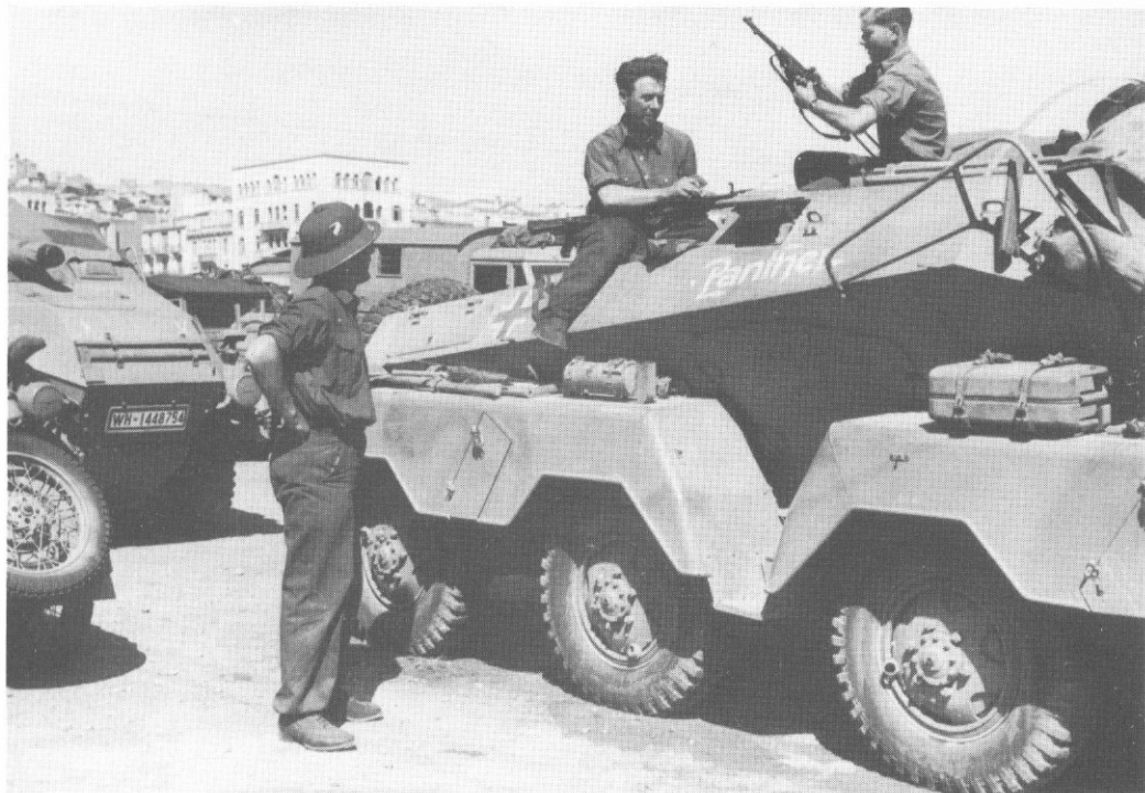
This and facing page 5th Panzer Division armoured cars in Greece: an SdKfz 232 ('Seydlitz') ( above ), 233 ('Panther') ( below ) and 221 ('Houx') ( right ) (163/327/24, 175/1265/14 and 164/369/29a).
