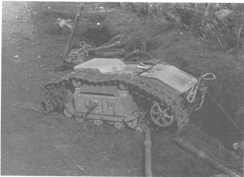
Above A disabled Goliath remote-controlled demolition tank (310/898/34).
